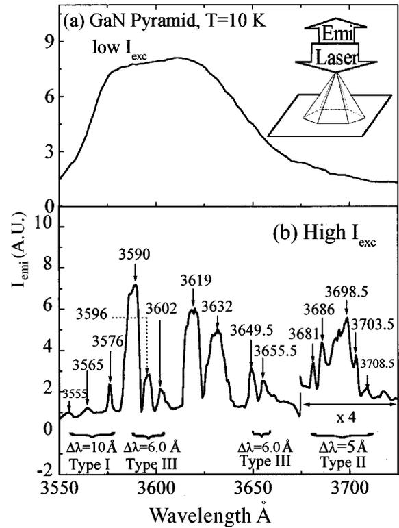
FIG. 2. (a) PL emission spectrum of GaN pyramids under a low pump intensity and (b) optical resonance modes behavior of an individually pumped pyramid under a high pump intensity.
